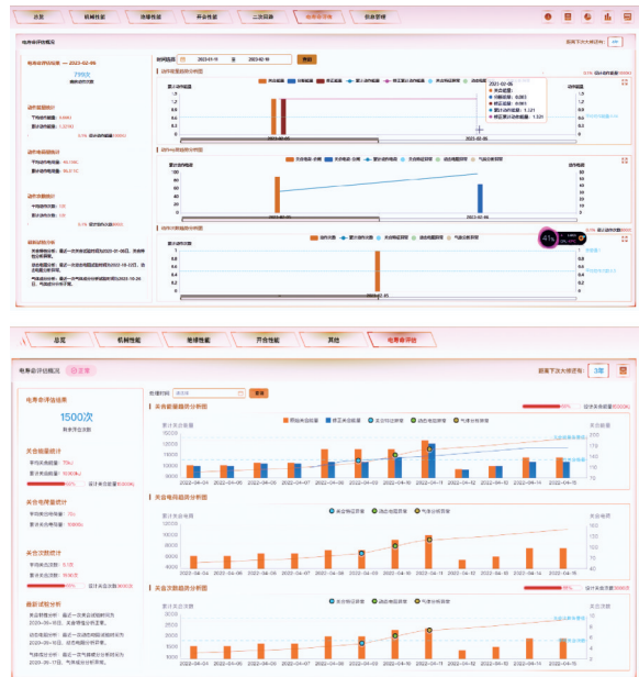
图18 滤波器组断路器电寿命评估系统 Fig. 18 Electrical life evaluation system for filter bank circuit breaker
